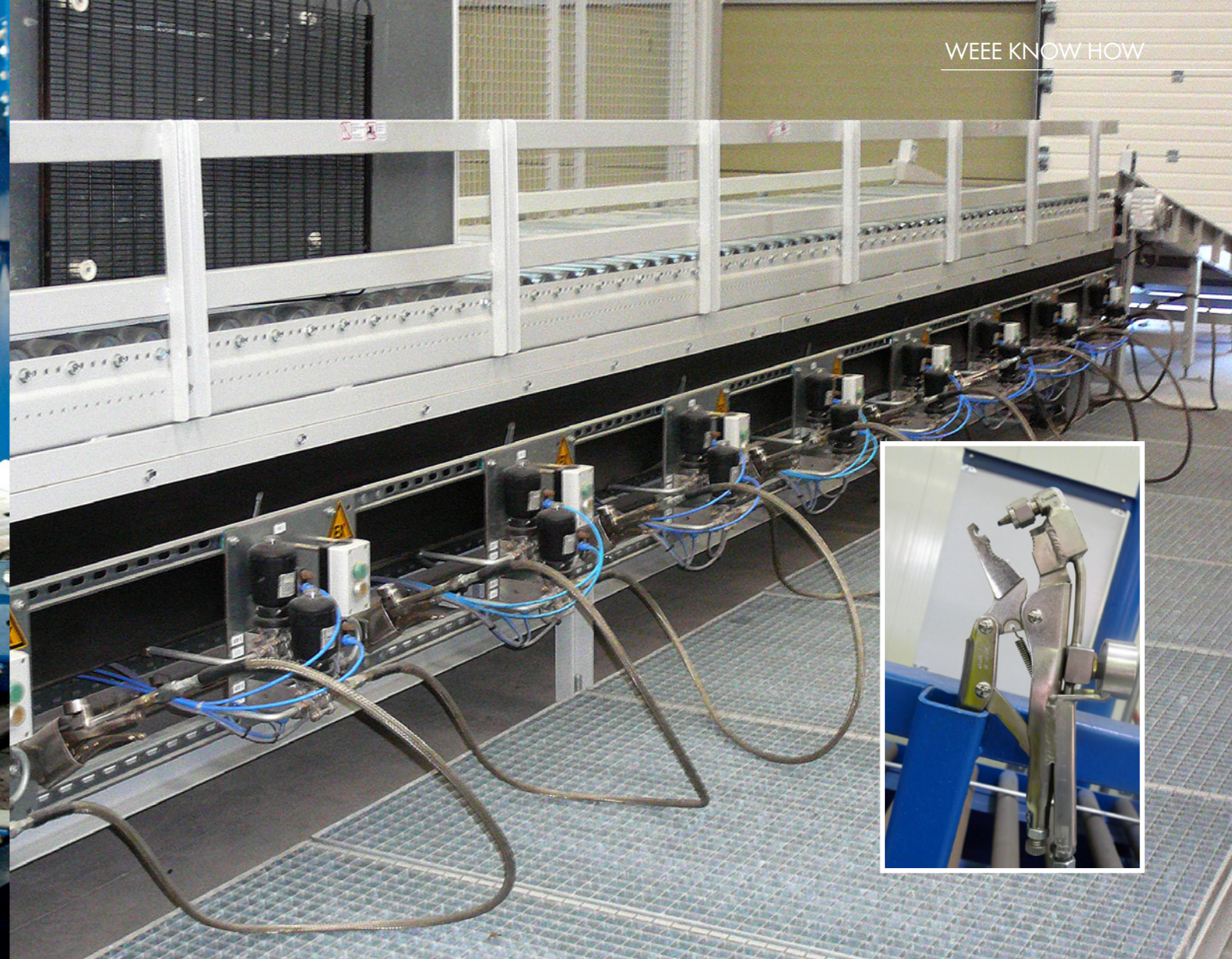
Step I plant with logistic line, piercing pliers and tilting table
