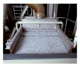
MSort covers visible sorting as well as the ability to detect materials using infrared spectrum and X-rays technology. Each of these technologies can be used to sort material according to pre-determined physical and chemical material properties.
